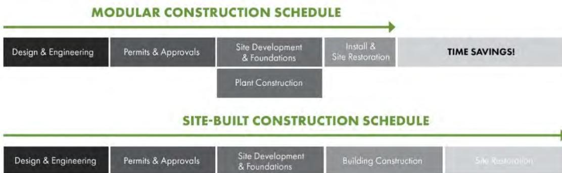
*Figure 13 – Modular Construction Schedule vs Site Build*
