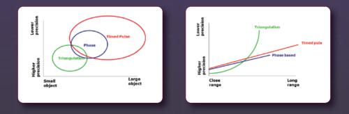
Each category of instrument has distinct and differing technical characteristics, so a surveyor needs to select the most appropriate device to optimise a survey.
